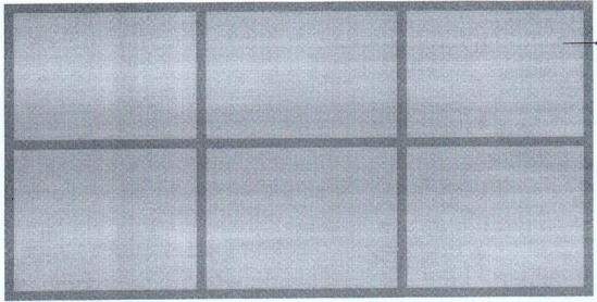
→ 20 gauge M S Sheel with edge folding on 50 x 6 mm bar
